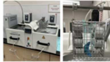
Figure 2. Thermocycler. The composite samples were artificially aged to mimic the conditions in the oral cavity for 1-month (833 cycles), 6-months (5,000 cycles), and 12-months (10,000 cycles). Set up of composite samples in the Thermocycler. Samples were fastened in the thermocycler with a floss and a putty to maximize composite contact with the water bath.
