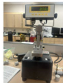
Figure 5. Ultratester was used to collect data of shear bond strengths of the composite buttons.
